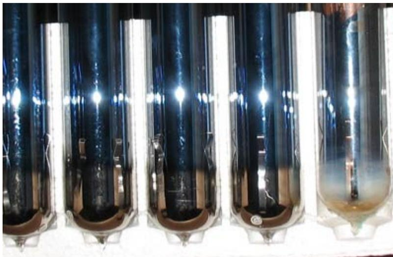
TIP! The silver surface at the base of the glass heat pipe is there to show that the vacuum is in tact. Any damage can be identified by the immediate loss of the silvering, indicating a need to replace the glass. Tubes are an industry standard product, spares are readily available from Solarproject, or any solar supplier.
