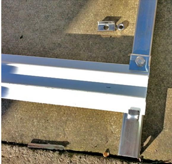
4/ Attach the alloy base bar using the 2 nut/bolt/washers\*, with the nuts and retainer facing you, on what will later be the underside of the frame. Finger tightness is sufficient at this stage. Note that the thicker lip of the bar faces upward (if applicable)
