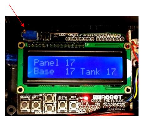
MANUAL PUMP - Manual Over-Ride switches pump on, while reporting the three Probe Temperatures.
