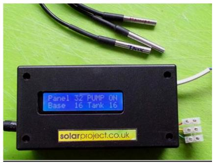
□ Low Voltage (6 to 14V DC) Solar Water Controller.
